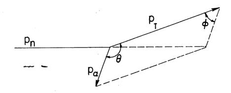
FIG I VECTOR DIAGRAMS SHOWING CONSERVATION OF LINEAR MOMENTUM IN THE (n,  $\alpha$ ) REACTION IN Li  $^6$
